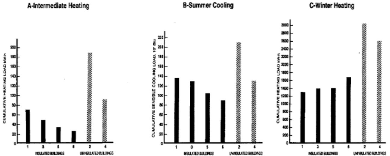
During this 3-week intermediate (spring/fall) heating season, the log building #5 used 46% less heating energy than the insulated wood frame building #1.
